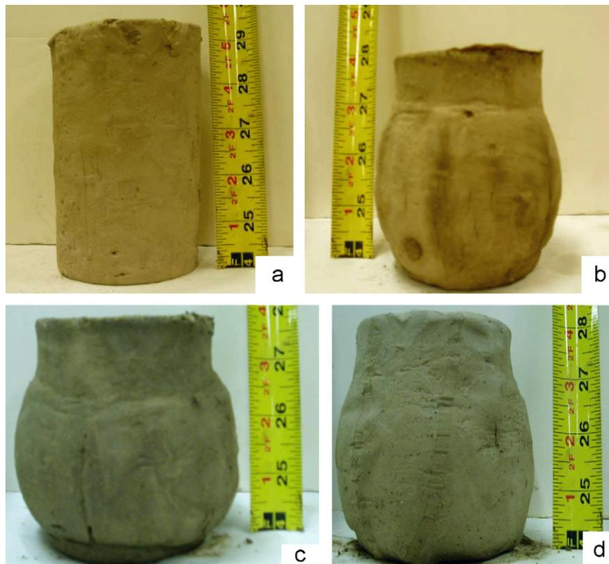
Fig. 7. Photographs of CTC test samples: (a) before the test; and (b), (c), (d) after test; (b) for Sky Pilot; and (c) and (d) for Tiskilwa Till.
