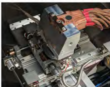
The custom EBSD holder with flexible Cu braid provides heating and cooling of large ice samples down to -160 °C.
