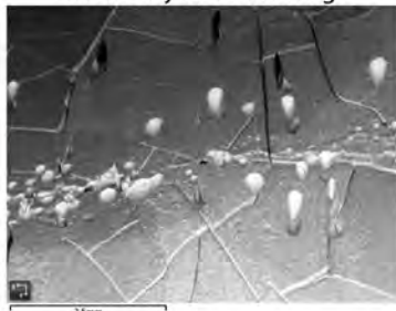
Electron images acquired from the surface of a polished ice sample at -85 °C and 26 Pa chamber pressure reveal bubbles in the ice and cracks in the sample surface.
