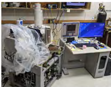
The “Ice SEM” in room 318 consists of large chamber SEM, LN dewar with cryo stage attachment, purgable glove bag with O 2 sensor, and associated detectors.
